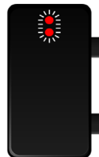
Indication for LAA Calibration (Red LEDs Flashing)
